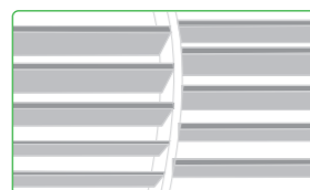
All vanes are dislocation distribution to offset sound wave, so that the noise can be reduced.
